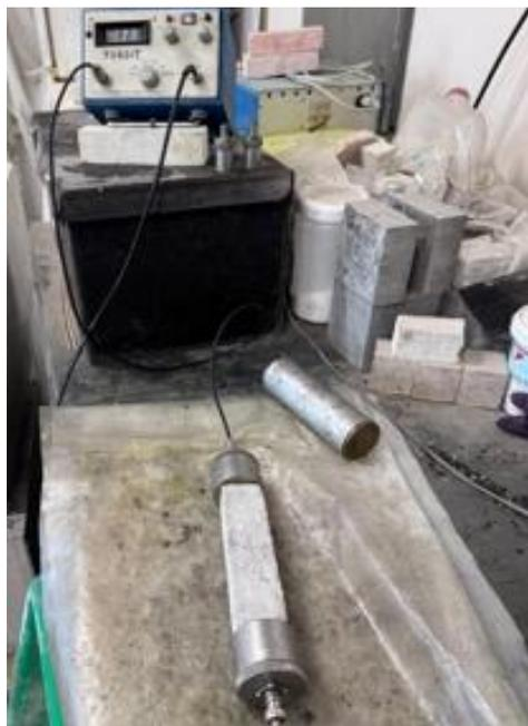
Figure 4. Ultrasonic pulse velocity test illustration
