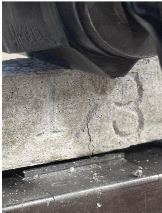
Figure 3. Tensile test strength using flexural loading
